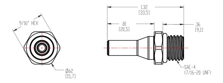
Description: 1/4" Rack and Panel SAE-04 Valved In-Line Liquid Cooling Coupling Insert
