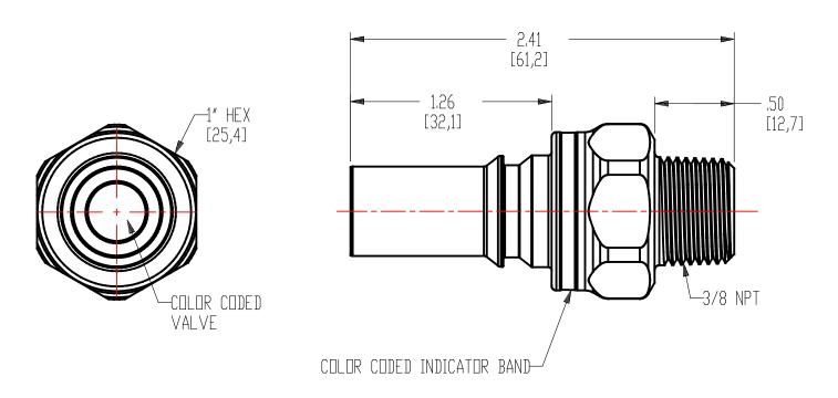
Description: 3/8" NPT Valved IN-Line Liquid Cooling Insert, Cool Blue
