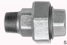
UNION TAPER SEAT BSPT MALE / BSPP FEMALE
