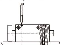
Fixation of screw at bottom surface
