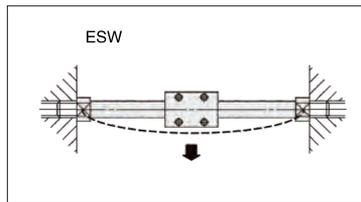
Note: Please reserve clearance according to the self-weight downward bending range shown in the right figure to prevent the cylinder from touching the installation surface or the load, so that the cylinder can slide smoothly within the minimum pressure range.
