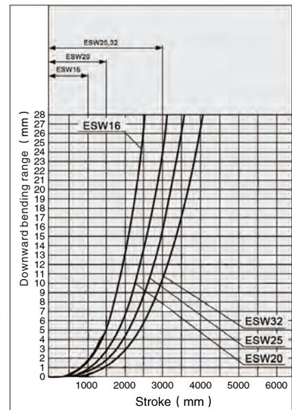
Note: the data of downward bending range is measured when the external slider moves to the middle of the stroke.
