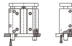
Fixation of T slot at bottom
