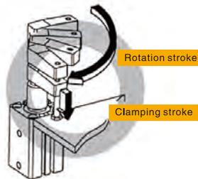
10. The installation method as the diagram below is wrong, and will injure the cylinder and shorten the cylinder life.
