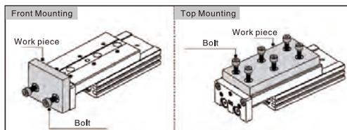
2.2 When mounting a work piece, tighten the bolts properly at a torque value within the limiting range. Use bolts at least 0.5mm shorter than maximum thread depth to prevent bolts from contacting the guide block. If the bolts are too long, they hit the guide block and cause damage.
