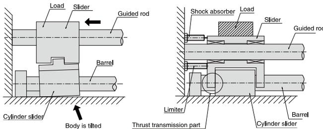
5. (4) In a vertical installation situation, a pneumatic circuit cannot be used to stop the cylinder. Piston stopped because of pressure increase, but the magnetic coupling is at risk of demagnetizing due to the weight and inertia of the load.
