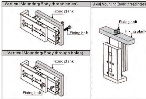
1.2 When mounting an compact slide cylinder, screws of appropriate length should be used and tightened properly within the maximum tightening torque. If screws are tightened beyond designed limits, malfunction may occur. If they are tightened insufficiently, it may result in sliding or falling off from its position.
