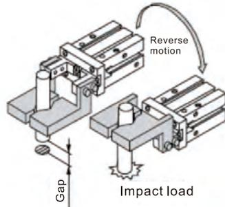
9. When ripping an object the item should always be centred. When testing, you must reduce the pressure for low speed running, to guarantee the safety and no impact.
