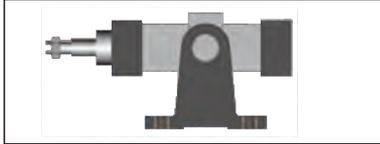
11. Proper installation shall be adopted considering the direction of load (flange type installation).
