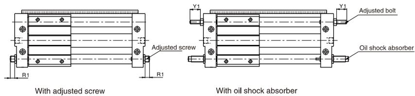
Note: Both sides tubing and central tubing have the same stroke adjustment.
