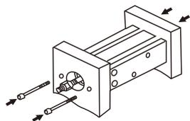
Vertical-shaft model (with through bore in the body)
