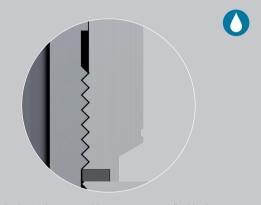
The lock nut has a marking groove on cylindrical Whitworth tube threads.
