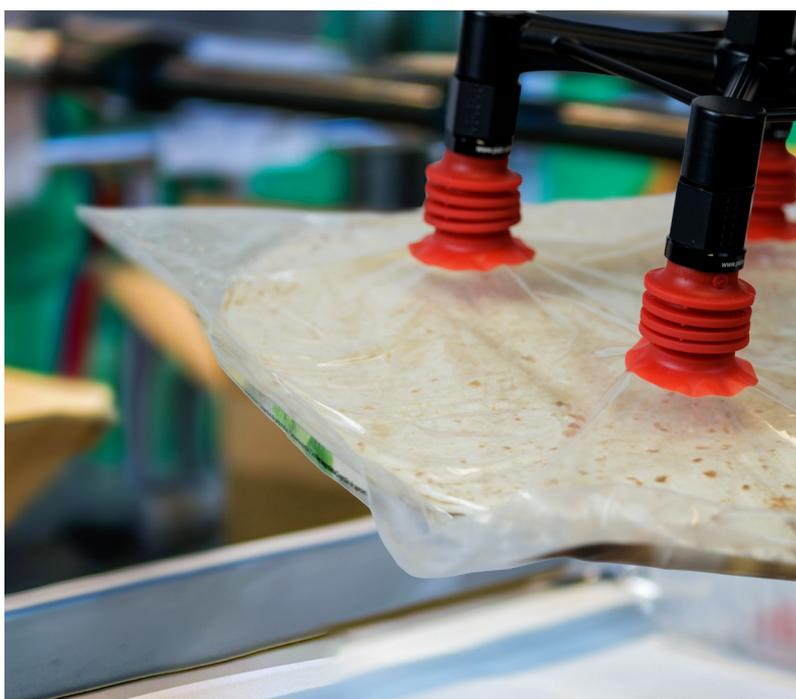
The BL-4 cup is designed for bags with fragile content such as snacks or frozen food. To suit this application, it is equipped with a longer lip and cleats.
