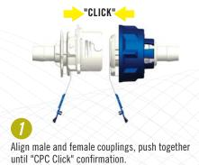
Slight rotation of lock ring may be required for proper alignment prior to connection.
