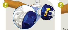
Twist the blue lock ring clockwise until audible "CPC Click." Alignment of the lock ring rib with the body's arrow indicator confirms final connection.
