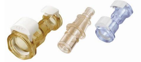
**MPC/MPX Back-to-Back Adapters** give end users the flexibility of connecting single-use systems that feature identical coupling connections at the end of their tubing. Combining both MPC and MPX couplings provides a reducing option for users who need to transition between tubing diameters ranging from 1/8" to 1/2".
