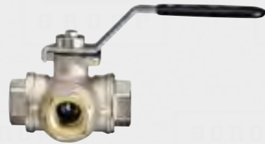
Three way full bore valve. Female threaded. T/L Port, with steel handle and ISO 5211 pad for actuator.
