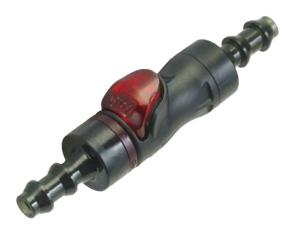
Everis<sup>TM</sup> PLQ2 Nominal flow of 1/8" (3.2 mm) with a Cv of 0.37 (Kv 0.32) Termination options: Locking hose barb, SAE, G thread
