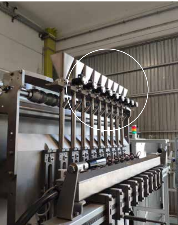
K (linear pneumatic vibrator) - Hopper emptying
