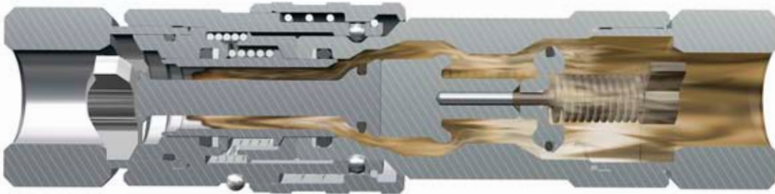
2 The coupling and nipple fully connected.
