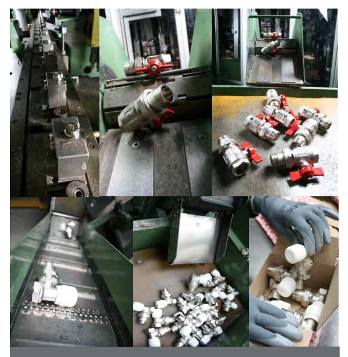
ITAP can count on 51 automatic assembly and testing lines; every day about 200,000 valves are fully assembled, tested and delivered to the storage warehouse and made ready for dispatch.
