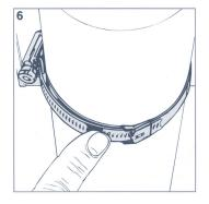
Push any remaining excess band through the buckle for a safe, tidy job. Tamtorque can be released and repositioned if required.
