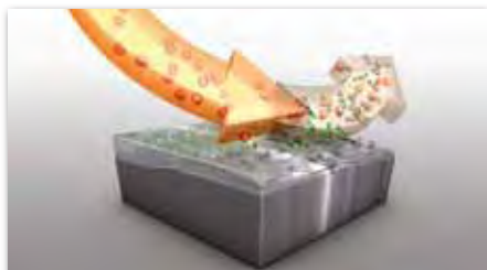
Small fillers knocked out by large particles
