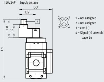
[4] Electrical connection M12x1 to ISO 20401 conforming to EN 61076-2-101, 4-pin version for connecting cable NEBU-M12
