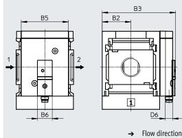
[AD11], [AD12] Pressure sensor with LCD display
