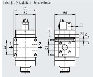
Retaining screw M6xmin. 90 to DIN 912 (not in the scope of delivery) for wall mounting without mounting bracket → Flow direction
