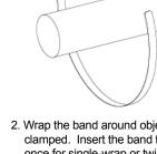
2. Wrap the band around object to be clamped. Insert the band through buckle once for single-wrap or twice for double-wrap. Double-wrapped clamps have more than 3 times the loop-tensile strength. **DO NOT FEATHER**
