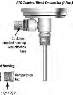
Type TT.30 w/RTD terminal block
