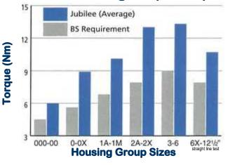
The performance of hose clips is determined by the hose type, spigot, tightening torque and hose working pressures - phone for technical advice
