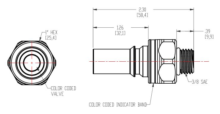
Description: 3/8" SAE Valved In-Line Liquid Cooling Insert, Cool Blue
