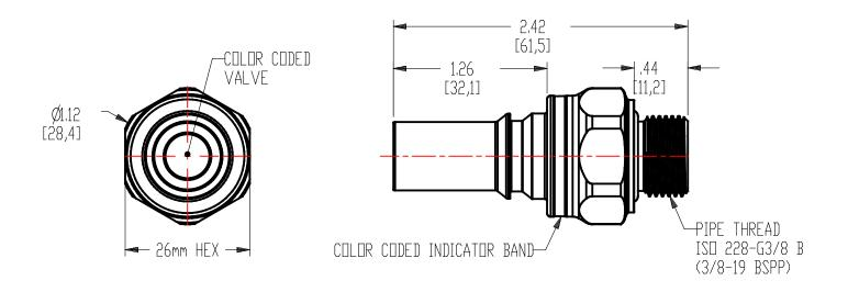
Description: 3/8" G-Thread/BSPP Valved Liquid Cooling Connector Insert, Cool Blue
