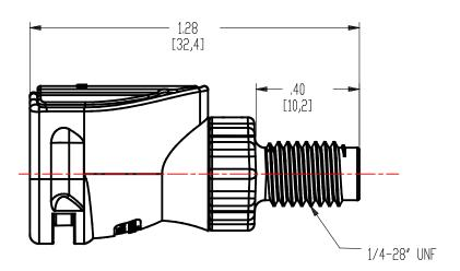
**Description:** 1/4-28" Male Thread Valved In-Line Coupling Body
