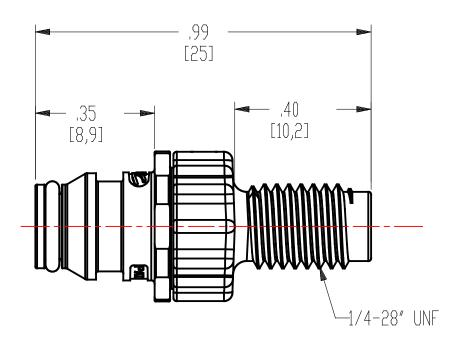
**Description:** 1/4"-28 Male Thread Valved In-Line Coupling Insert
