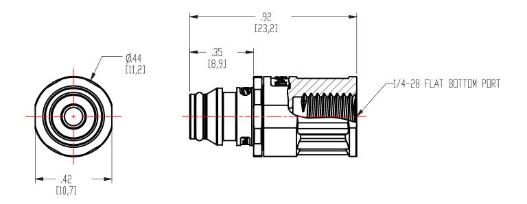
**Description:** 1/4"-28 Flat Bottom Port Valved In-Line Coupling Insert
